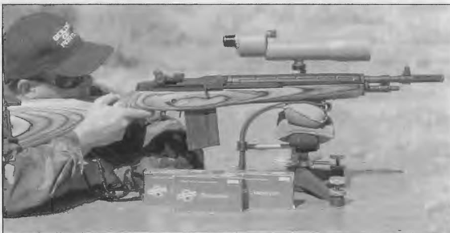
Test-firing the Springfield Armory M1A-A1 Bush Rifle for accuracy from the bench.
